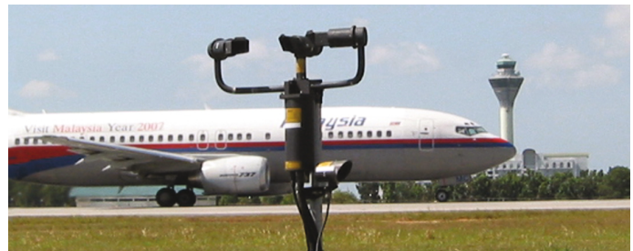
VPF sensors were the first forward scatter sensors to be used in a UK CAA approved RVR system on a CAT III runway.
